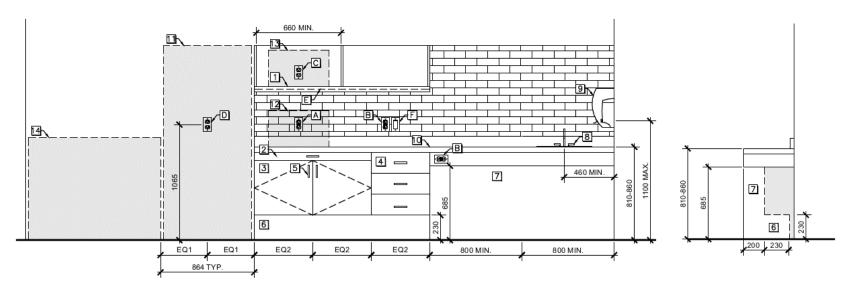
The included dimensions are taken from the CAN/CSA B651 Accessible design for the built environment - Please refer to clauses referencing Kitchens for all CAN/CSA B651 requirements.
